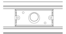
STEP 2: Remove a knockout for connection to appropriate Chicago Plenum rated conduit (by others). Make the necessary electrical connections inside the junction box and screw the cover on using (2) screws (provided).
